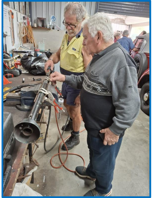
Jim Whately and Dan Fanetti working on the steering column
